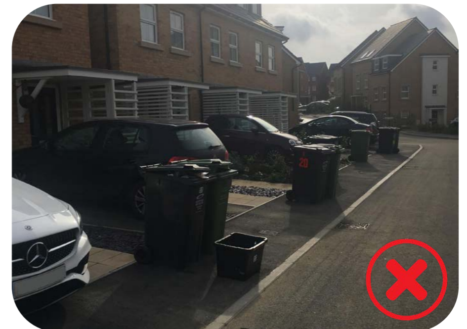
Avoid Long Lines of Unbroken Driveways and Ensure Suitable Driveway Length, Phoenix Quarter, Dartford
